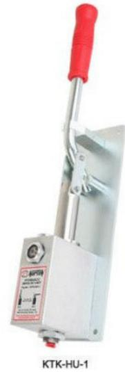
KURTEK Hydraulic Control Unit is used to close Quick Closing Valves in the fuel supply line of each engine and generator. For hydraulic remote control, KURTEK Quick Closing Valve is equipped with a hydraulic cylinder which is activated by a special single piston impulse unit.
