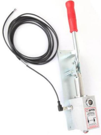
KURTEK Hydraulic Control Unit is used to close Quick Closing Valves in the fuel supply line of each engine and generator. For hydraulic remote control, KURTEK Quick Closing Valve is equipped with a hydraulic cylinder which is activated by a special single piston impulse unit.
